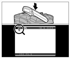
Close the flash to switch to Suppressed Flash mode.
